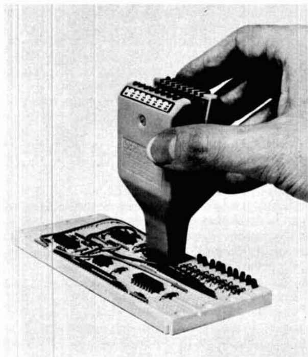
Continental Specialties Logic Monitor LM-1 facilitates checking digital ICs and associated circuits. Priced at $84.95 from Continental Specialties Corporation, 44 Kendall Street, Box 1942, New Haven, Connecticut 06509.
